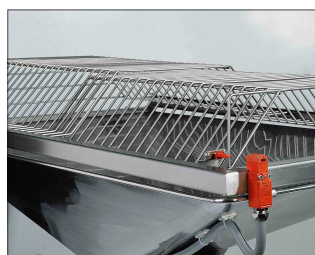
HLR hopper with sliding grid
