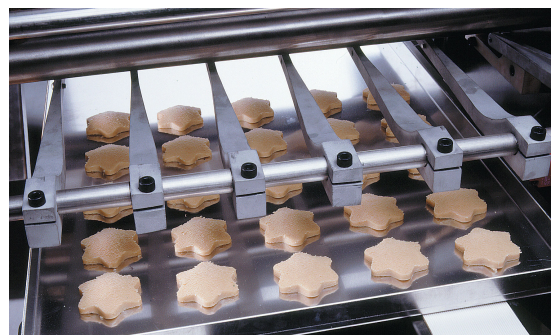
Operation with wire cut system
