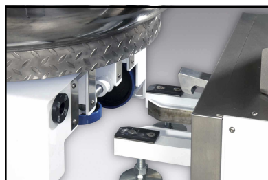
Trolley coupling to the machine unit
