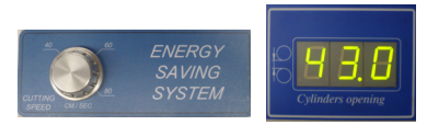
Electronic variation of the belt speed and cylinders opening display (Luxe version)
