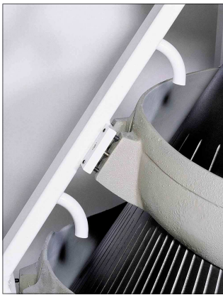
Conical rounder with "A" hot air blower
