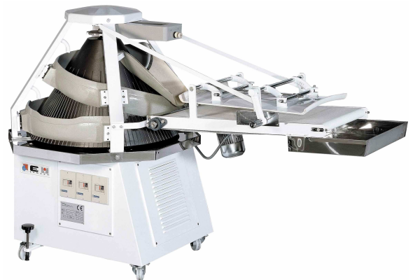
Conical rounder with "CF" long moulding device
